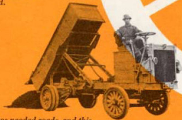
Autos needed roads, and this early GMC self-powered dump truck helped to build them. Note the air horn at the driver's right.
