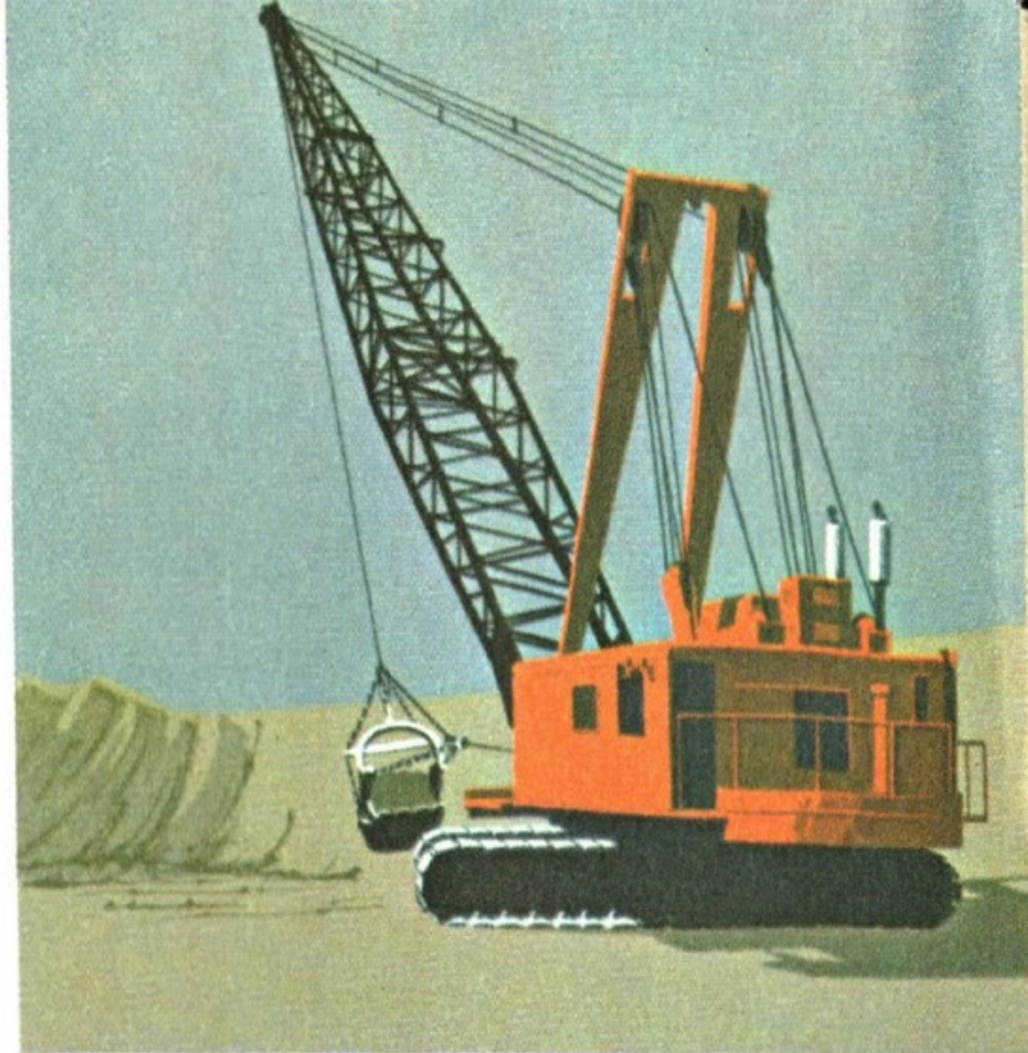
A 700 horsepower Detroit Diesel engine powers this huge dragline
