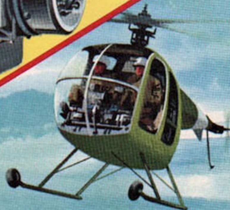
Allison powershift transmission; light helicopter using Allison T63 lightweight gas turbine engine
