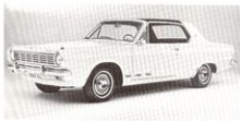
1965 DODGE DART GT: A 235-horsepower, 273-cubic-inch high-performance option was added to the Dart engine lineup for 1965. Two-door hardtops became available in the Dart 270 series, and vinyl roof covering was a Dart GT option. The lower-line Dart series offered all-vinyl seating fabric as standard equipment.
