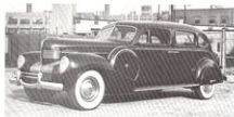
1939 CHRYSLER CUSTOM IMPERIAL, C-24: The first application of a fluid coupling to passenger cars in the United States was made late in 1938, when Chrysler introduced Fluid Drive as standard equipment on the Custom Imperial, C-24. Also new to all Imperials as standard equipment was the steering column-mounted gear shift lever.
