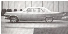
1963 DODGE CUSTOM 880: Now in its second year as a big-car Dodge, the 880 was dressed in new front end sheet metal. Over-all body length was increased by 1.3 inches and a 383-cubic inch engine with two-barrel carburetor and single exhaust system made available as a power option. Dodge (along with other Chrysler cars) introduced airfoil windshield wipers as standard equipment.
