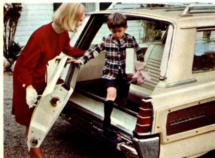
In this illustration, Mercury's tailgate is swung out as a rear passenger entrance and exit from the rear.
