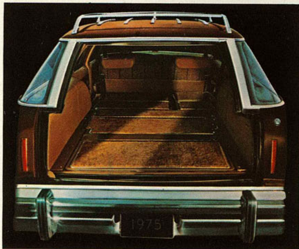
Above: The power operated window slides into the roof and the door glides under the load floor.
