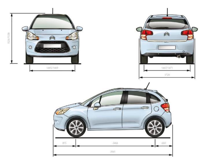
All measurements are in millimetres.
