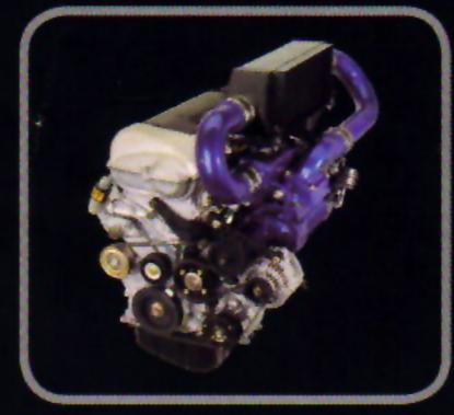
Engine: Toyota VVTL-i 2ZZ GE engine fitted with a supercharger and intercooler system.
