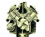
periodic adjustment. Valves spring and guides are assembled inte precision set units at the factory Valves are free-turning, they turn as they open and close, keep wear
