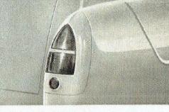
COMPACT TWIN TAIL-LIGHT ASSEMBLY . . . incorporates red stop light, amber flashing turn-indicator lights and built-in reflectors.
