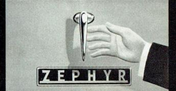
**CENTRAL TAILGATE HANDLE** allows easy, single-handed operation. The tailgate suspension chains are P.V.C. covered for load-protection.
