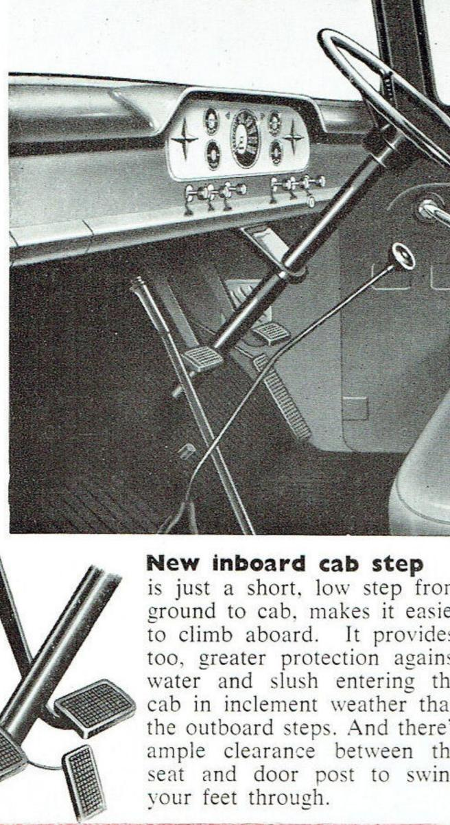
is just a short, low step from ground to cab, makes it easier to climb aboard. It provides, too, greater protection against water and slush entering the cab in inclement weather than the outboard steps. And there's ample clearance between the seat and door post to swing
