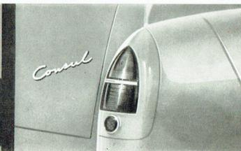
**COMPACT TWIN TAIL-LIGHT ASSEMBLY . . .** incorporates red stop light, amber flashing turn-indicator lights and built-in reflectors.
