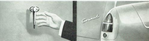
**CENTRAL TAILGATE HANDLE** allows easy, single-handed operation. The tailgate suspension chains are P.V.C. covered for load-protection.
