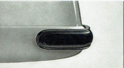
**REAR END PROTECTION.** Rubber-faced bumper-cets curve right around the vital rear corners, absorbs shocks better and do not show scratches.
