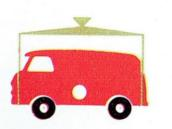
Even distribution of payload over the axles prevents damage to suspension system, ensures safe riding of load and gives perfect road-holding and stability even when fully laden.
