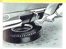
Ultra-fast wheelchange made possible by new-design carrier. Just raise the "Thames" nameplate, give a few turns of the wheel-nut wrench, and the spare wheel is resting on the ground Replacing the spare wheel is just as easy, takes only a few seconds.
