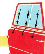
Sliding window panels of really big area give better weather sealing and ventilation control in the cab. Rainwater is directed by a concealed channel down the outside of the body skin, preventing inside rust.
