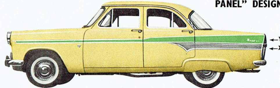
AR206E 19600 F "Ribbed Stainless Steel Panel" Moulding Kit is here combined with the AR206E 19600 D Fashionline mouldings—the effect is one of a painted upper portion—marked (Y), and a stainless steel lower portion—marked (X). Fender skirt A206E 18973 A is also illustrated. For Zephyr Sedan 1959/-.
