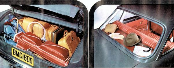
Capacious 17 cubic foot boot, free from spare wheel or fuel tank intrusion. Is equipped with automatic interior light. Other new lighting features include: pre-focused double-dipping headlamps; turn indicator flashers on wings as well as front and rear; day/night stop lights with variable brightness.
