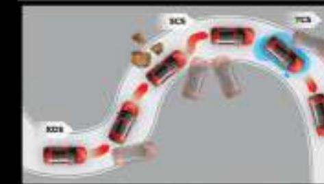
XDS (ELECTRONIC DIFFERENTIAL SYSTEM) SCS (STABILITY CONTROL SYSTEM) TCS (TRACTION CONTROL SYSTEM)
