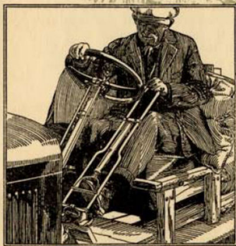
Measuring clutch pedal pressure
