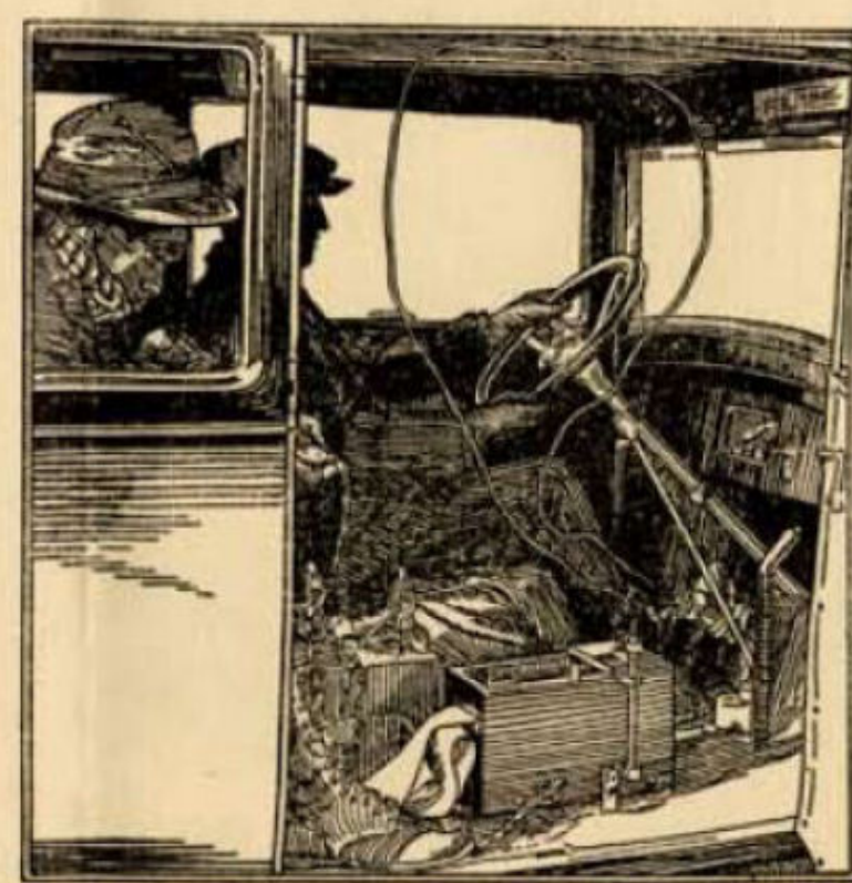
Measuring brake pedal pressure and deceleration
