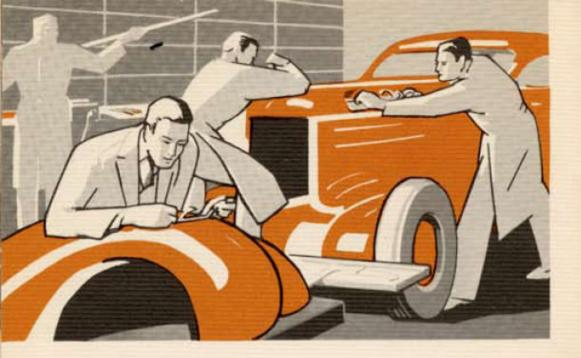
When the design has been accurately reproduced in clay, the activity shifts to the wood and metal shops. Here, as shown in the illustration, a new full-size model is built up out of mahogany and poplar. Metal parts, such as bumpers, grilles and body hardware are made by hand by skilled workers, and are finished complete down to the smallest detail and even plated with chromium where required.
