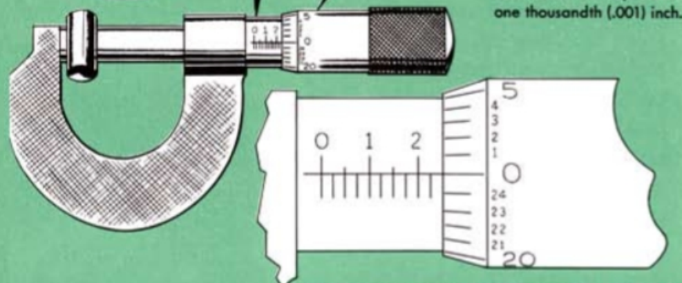
this micrometer setting is 250 thousandths (.250) inch.
