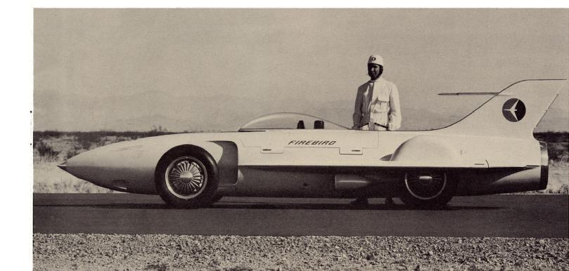
The aircraft motif is evident in the car's "needle" nose, delta wings swept back along the rear half of the body, a vertical tail fin and a plastic bubble over the driver's cockpit.
