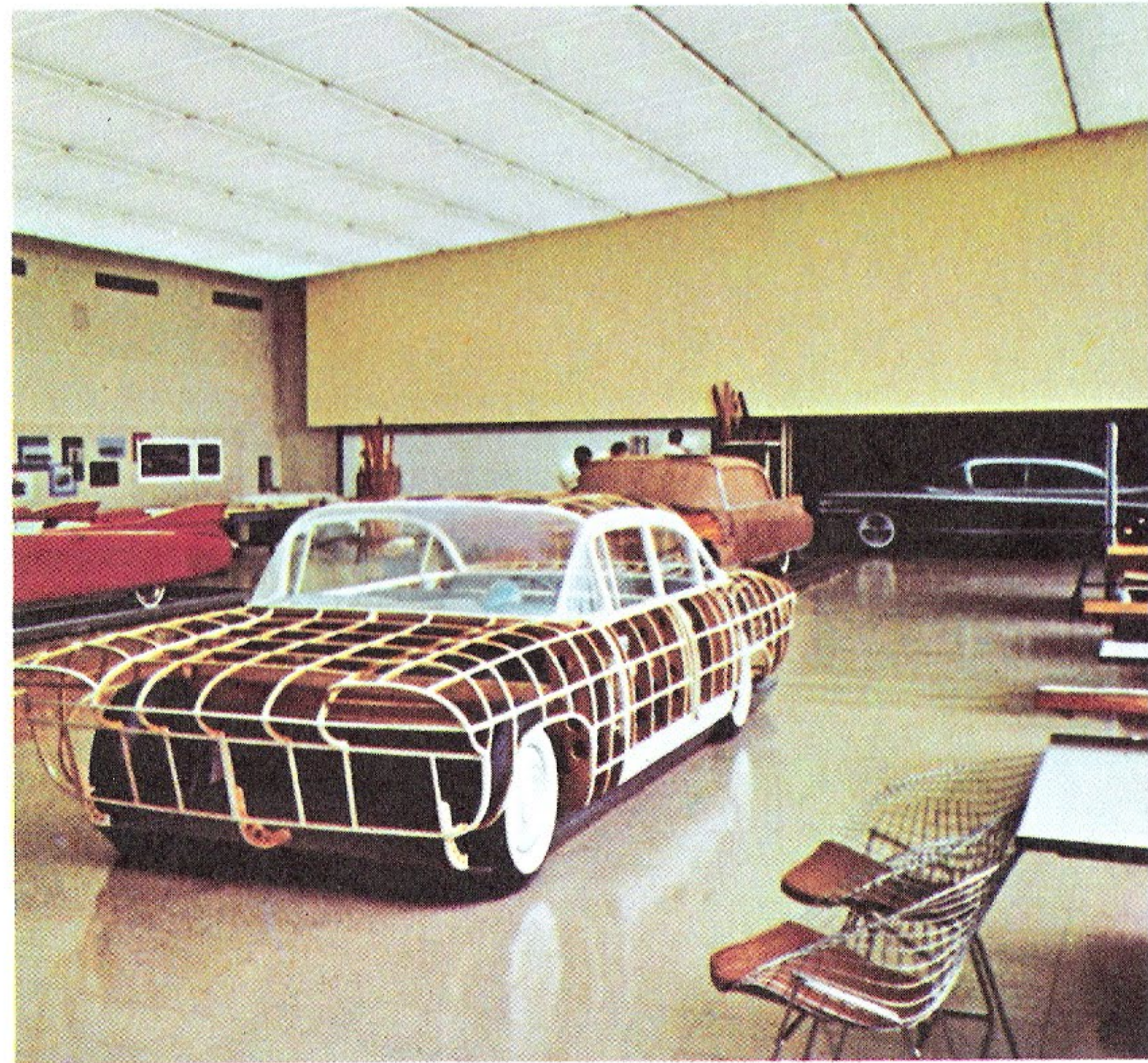
Automotive exterior styling is developed in sketches, mockups, clay models and fiberglass prototypes, in separate studios for each division.
