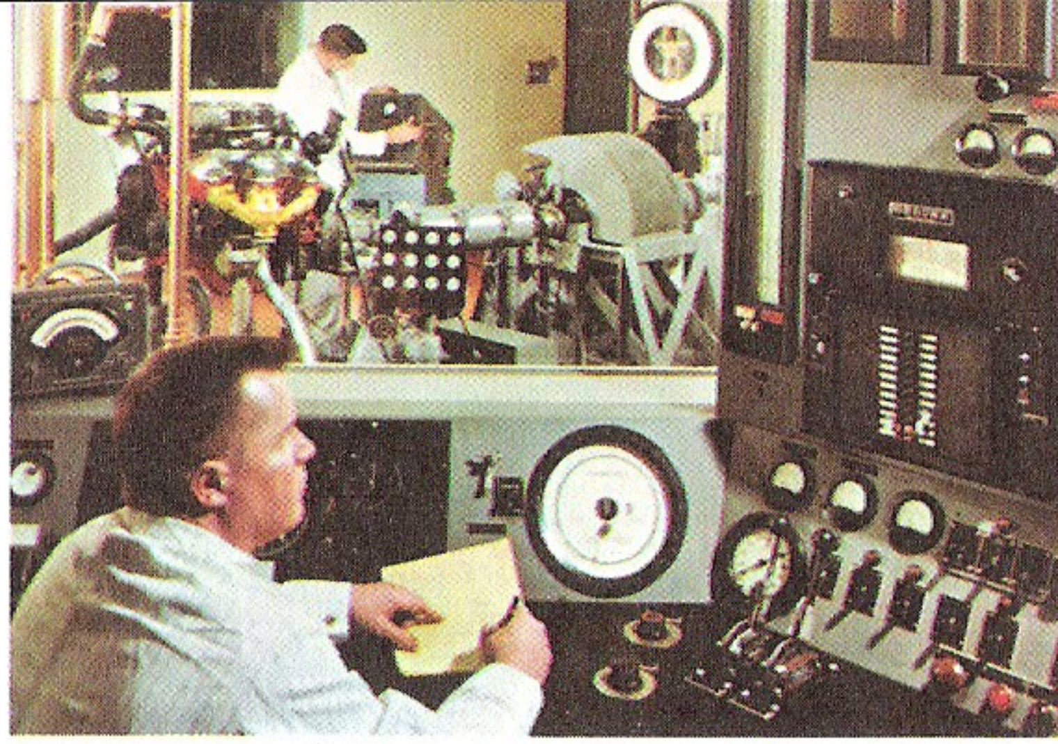
Engine tests in this dynamometer cell simulate on-the-road operation.
