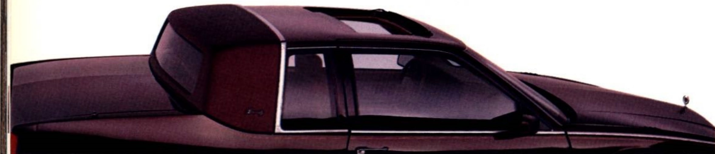
Standard formal cabriolet padded roof with opera lamps for Eldorado Biarritz. Shown with available Astrorooft 1 (reduces headroom slightly)
