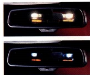
The standard Electrochromic inside rearview mirror automatically darkens to reduce glare.
