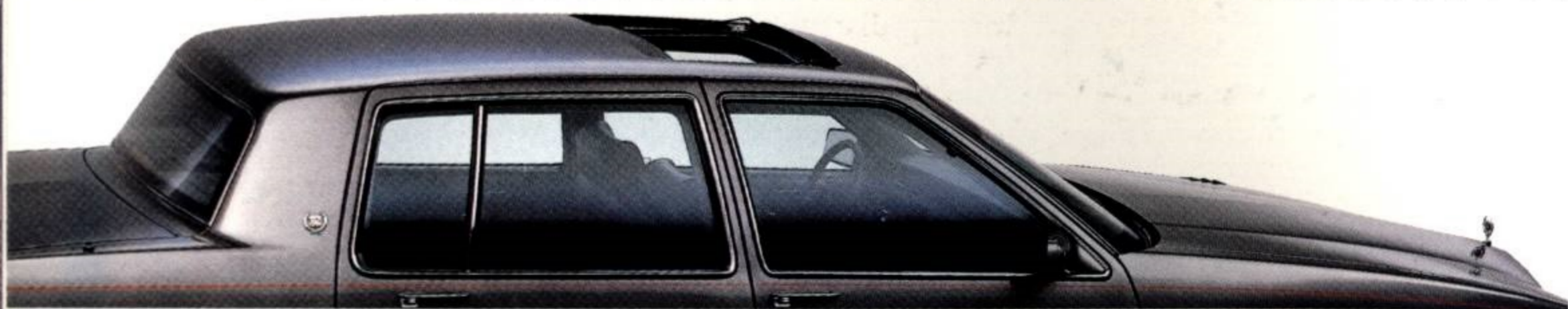
• Available express-open Astrorof (now available on Fleetwood Sixty Special); shown with available painted metal roof (reduces headroom slightly)
