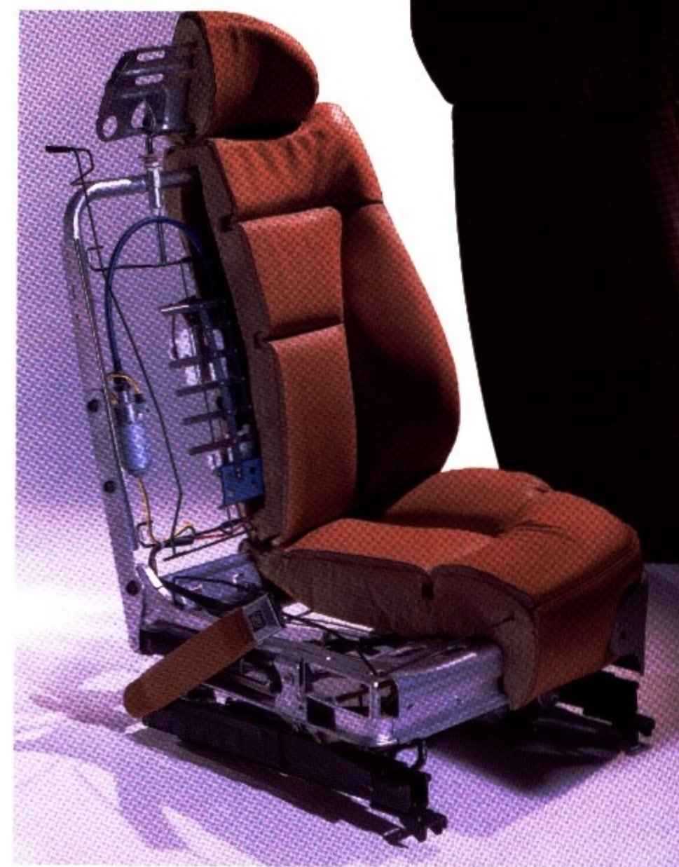
THE NEW DESIGN OF THE SEVILLE STS FRONT SEATS OFFERS DUAL-SPRING ACTION SUPPORT, PLUS POWER LUMBAR SUPPORT.
