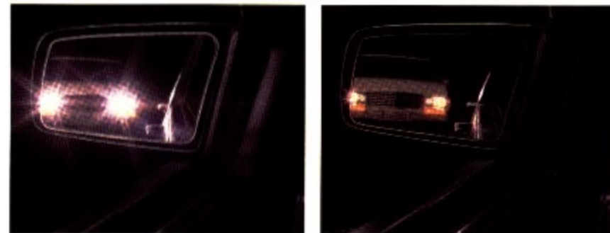
ELECTROCHROMIC OUTSIDE DRIVER-SIDE REARVIEW MIRROR DARKENS AUTOMATICALLY TO REDUCE GLARE.
