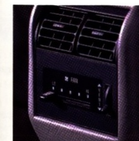
REAR ELECTRONIC CLIMATE CONTROL VENT.
