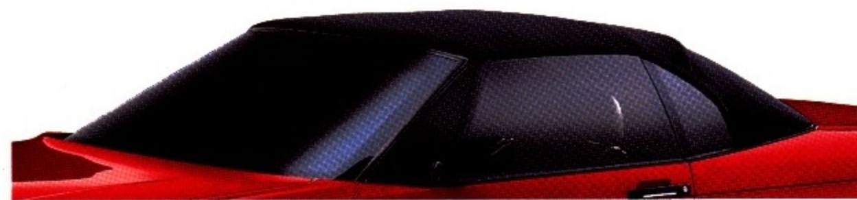
ALLANTÉ'S POWER-LATCHING SOFT-TOP DESIGN FEATURES GAS-STRUT ASSIST, ELECTRICALLY HEATED GLASS REAR WINDOW AND GLASS QUARTER WINDOWS.
