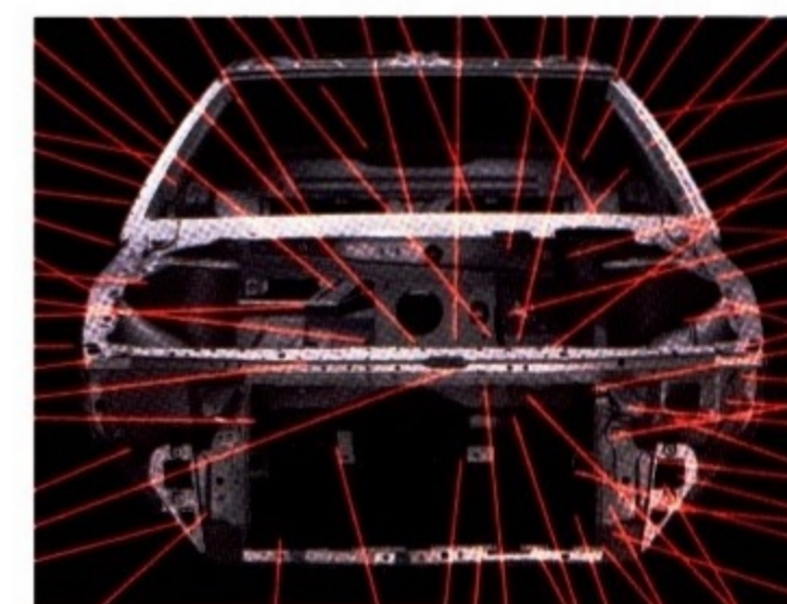
PERCEPTION SM LASER BEAMS PROBE AND PEER INTO CADILLAC BODIES AT MORE THAN 600 POINTS, VERIFYING ADJACENT BODY FITS THAT MEET YOUR EXACTING STANDARDS.
