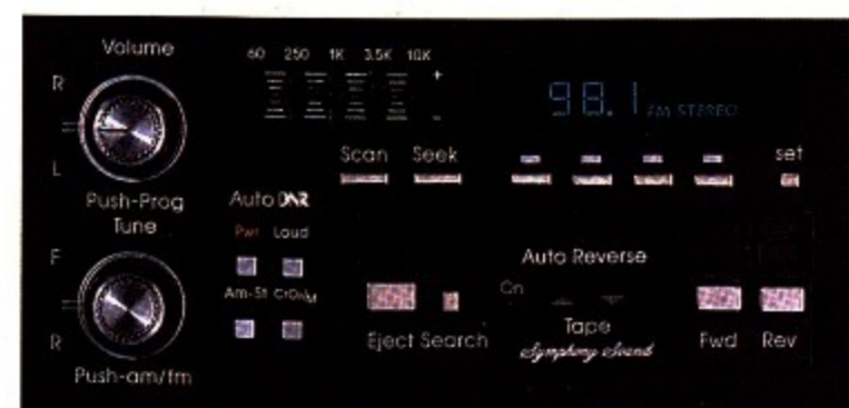
FLEETWOOD AND DE VILLE STANDARD PREMIUM AUDIO SYSTEM. SEEK/SCAN AM STEREO*/FM STEREO RADIO AND FULL-FEATURED AUTO-REVERSE CASSETTE TAPE PLAYER. FIVE-BAND GRAPHIC EQUALIZER.
