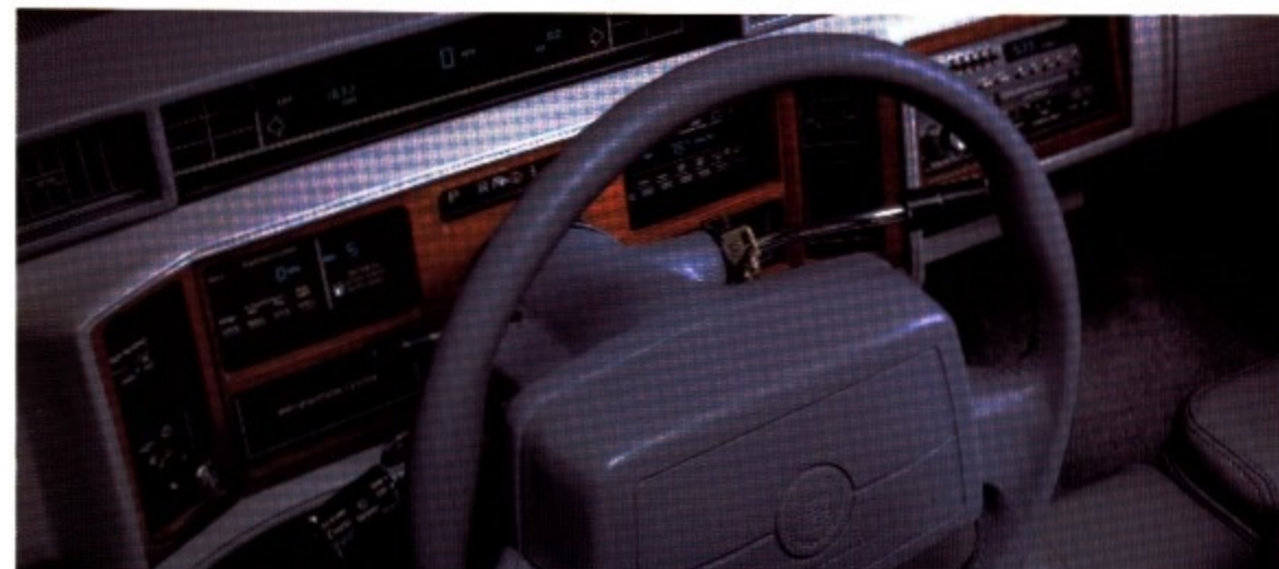
AN EASY-TO-READ DIGITAL INSTRUMENT PANEL LETS YOU MONITOR CRITICAL DRIVING SYSTEMS AT A GLANCE. THE STEERING WHEEL HUB CONCEALS A STANDARD SUPPLEMENTAL INFLATABLE RESTRAINT.
