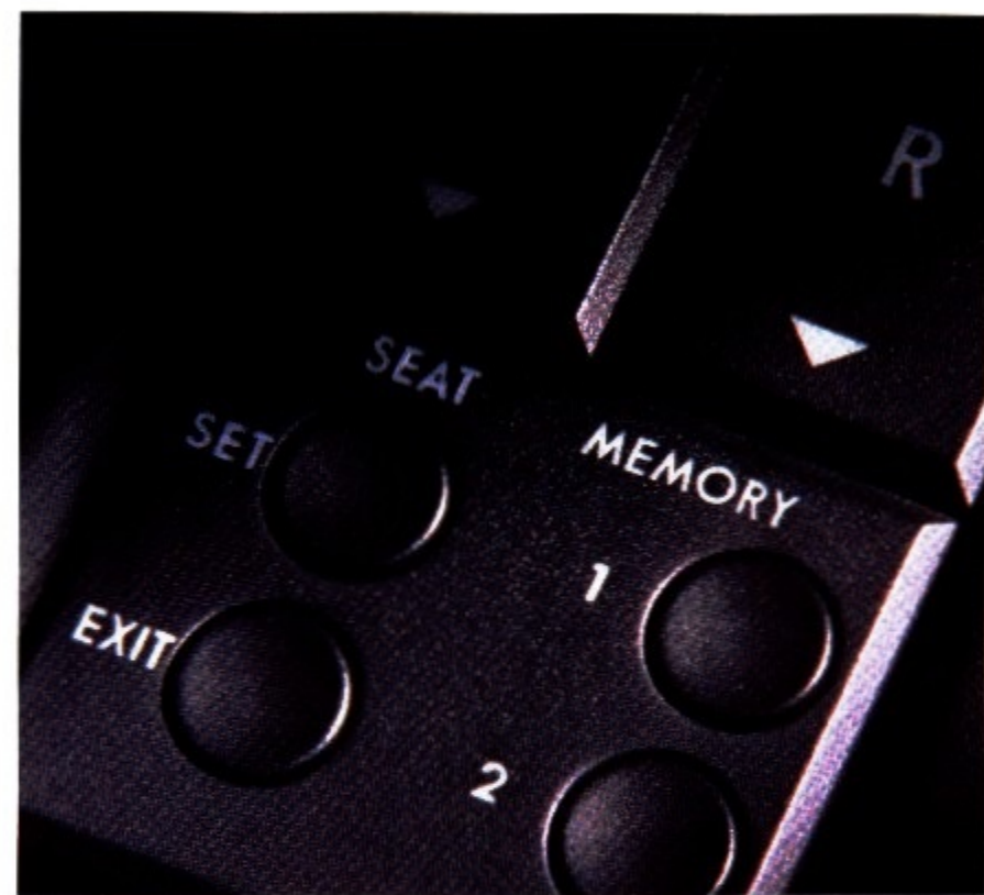
A DRIVER'S-SEAT MEMORY RECALLS TWO PREFERRED SEATING POSITIONS AND A PROGRAMMABLE EXIT SETTING.
