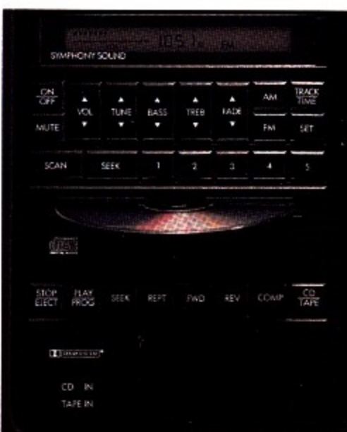
STANDARD BROUGHAM PREMIUM AUDIO SYSTEM INCLUDES FULL-FEATURED DOLBY ® B AUTO-REVERSE CASSETTE TAPE PLAYER AND SEEK UP/DOWN, SCAN UP/DOWN AM STEREO*/FM STEREO RADIO. FIVE AUTOMATIC TONE-CONTROL PRESETS.
