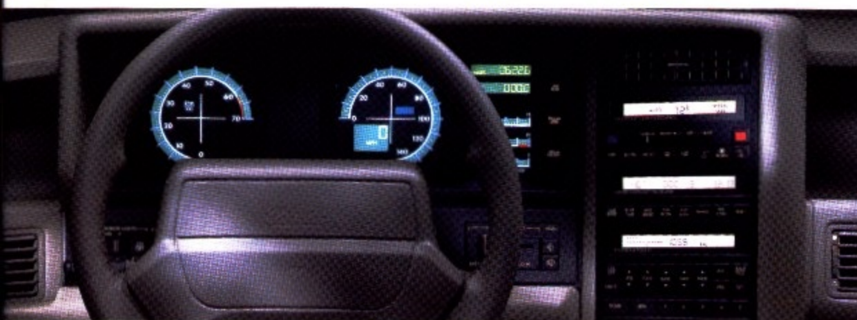
▲ Digital instrumentation, featuring liquid crystal displays, is available on the Allanté.
