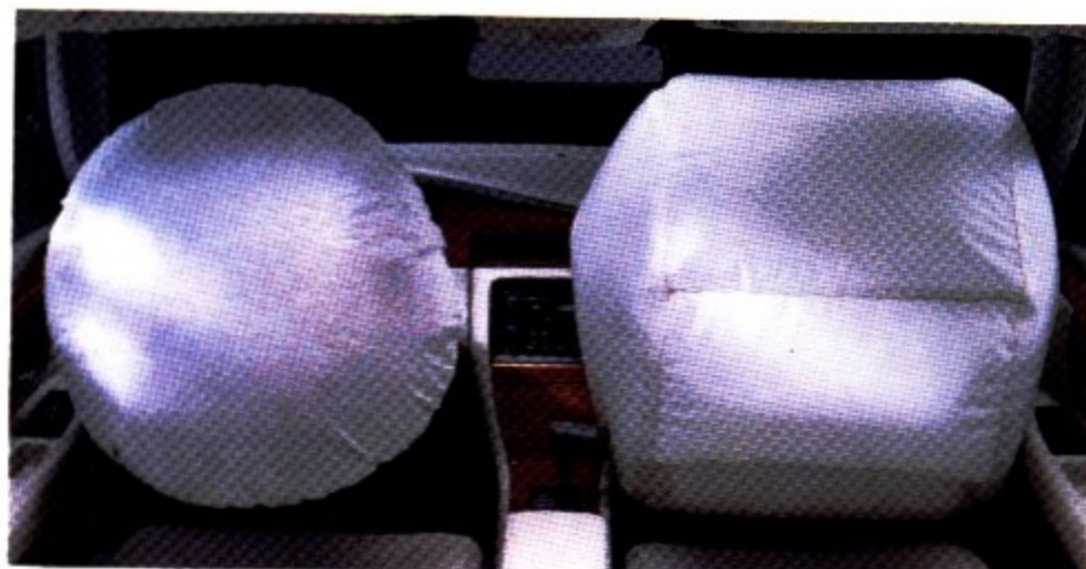
Designed to be used with the safety belt system, the driver- and passenger-side air bags increase your level of safety in less time than it takes to blink an eye.
