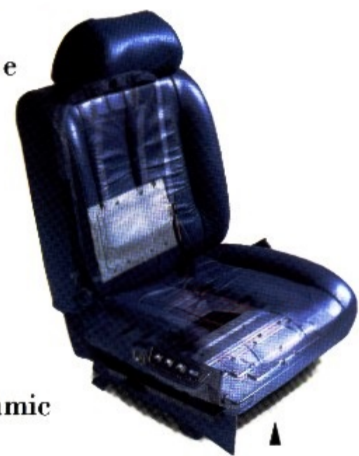
▲ Fleetwood Brougham's orthopedic front seats include triple-element lumbar supports, and are heated to relieve the chill of cold-weather driving.
