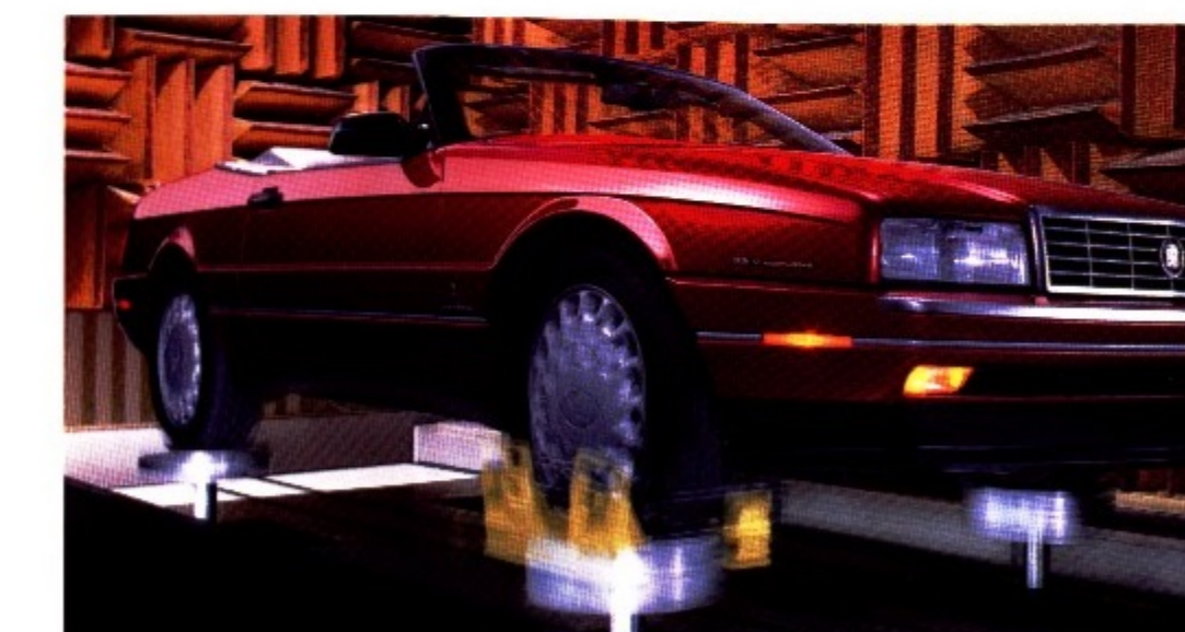
This road simulator dramatically shows how Road-Sensing Suspension isolates the Allanté from major road disturbances.
