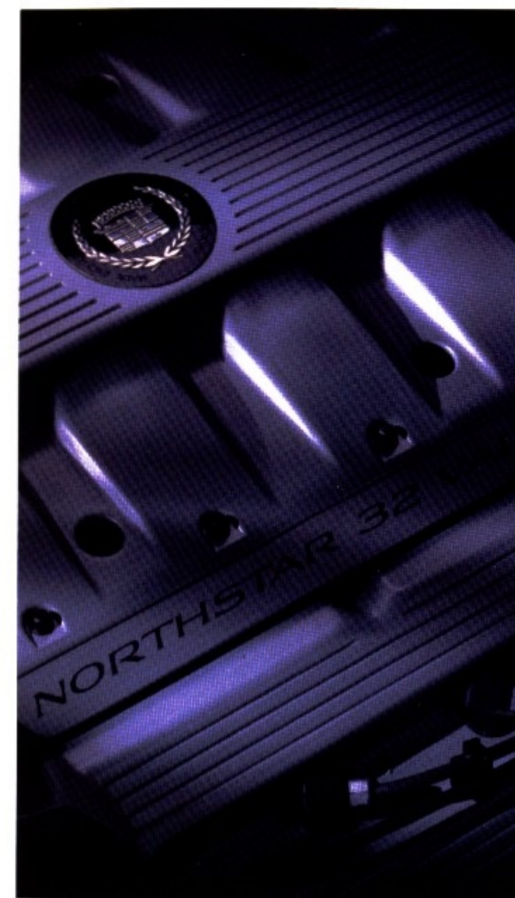
This 295-hp, 4.6L, DOHC 32-valve Northstar V8 requires its first scheduled tune-up at 100,000 miles, except for normal fluid and filter replacement. Its design created the need to refine every driving system to effectively apply this spirited power to the road.
