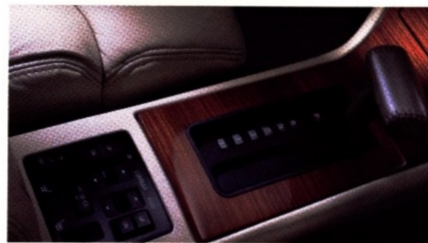
▲ The console on the Eldorado Touring Coupe houses lumbar support controls that let you adjust the support to the exact height and depth you require for optimum back support.
