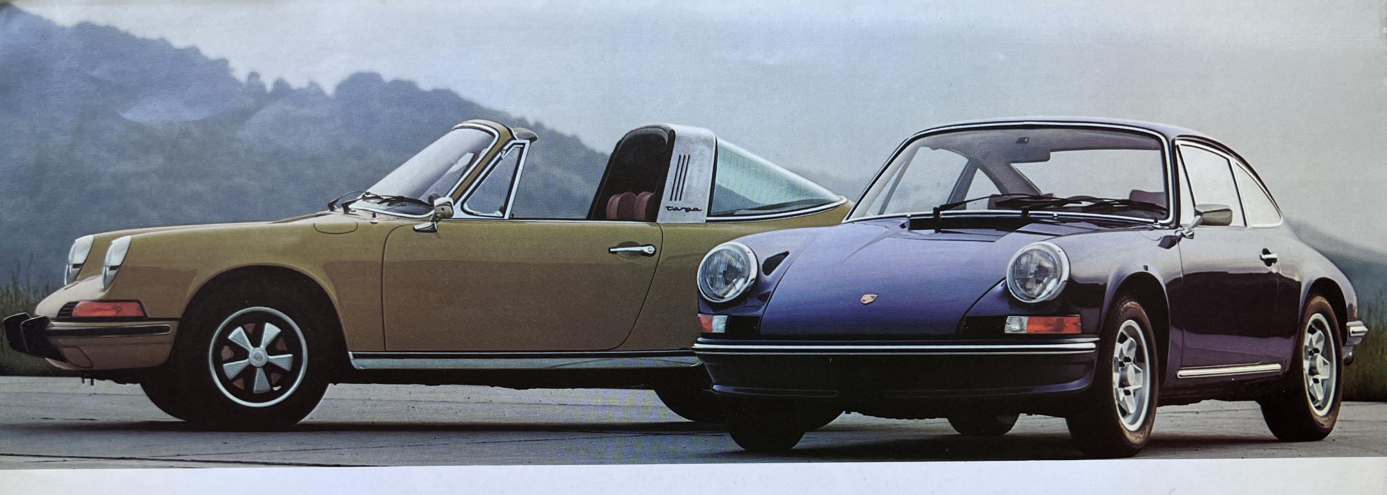
The Porsche 911 is available in three models; the 911 T with 135 DIN Hp (129 SAE net), the 911 E with 165 DIN Hp (157 SAE net) and the 911 S with 190 DIN Hp (181 SAE net). All three engines have a displacement of 2.4 liters and are fed by Bosch mechanical fuel injection. The engine is positioned at the rear for especially good traction under all driving condi-
