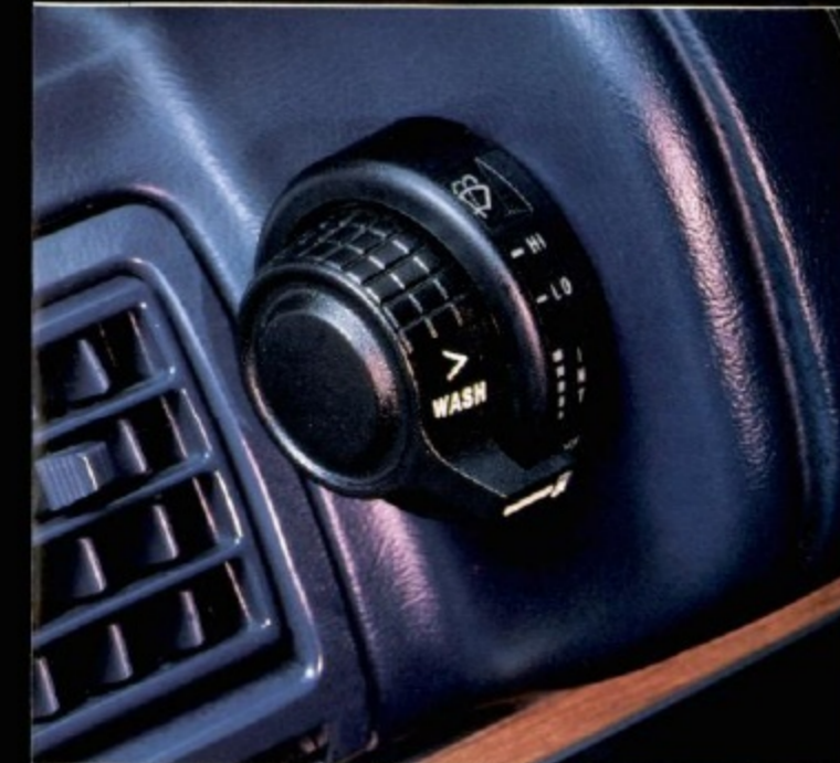
Windshield wiper/washer switch has been designed to allow operation without making visual contact. It is located on the left side of the instrument pod.
