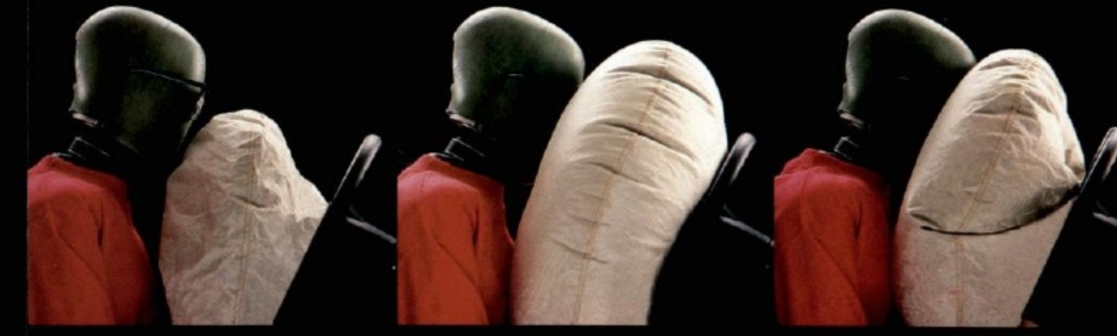
Optional Driver Air Bag Supplemental Restraint System. Laboratory testing has shown the supplemental driver air bag, combined with properly used safety belts, can provide extra protection against chest and face injuries that might occur in severe front-end impacts. It is so fast that it inflates in approximately 40 milliseconds. It is a proven system that has been field tested in thousands of cars driven millions of miles. To this date, not a single case of accidental air bag deployment has been reported by users. It is now available as an option on all four-door Topaz models. (Airbag deployment sequence shown here was not made during an actual test.)
