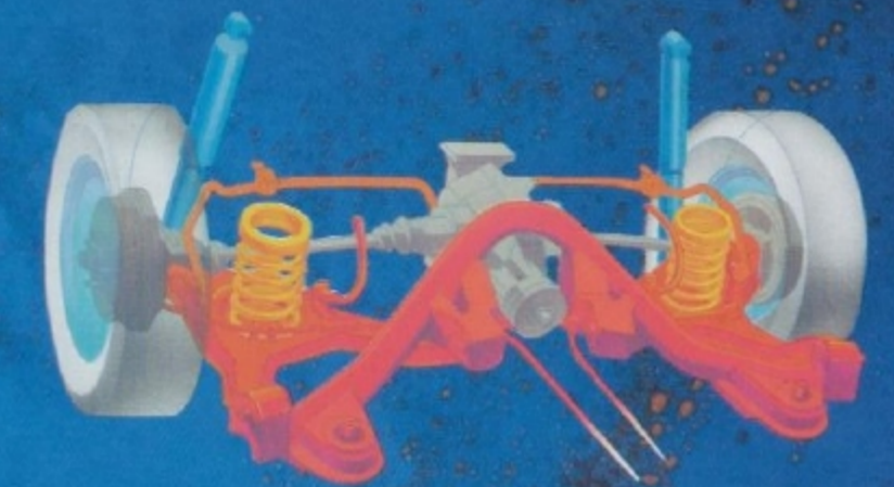
Independent semi-trailing arm rear suspension.
