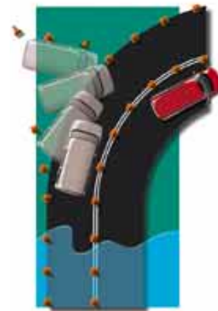
Four-wheel anti-lock brakes can help keep accidents from happening. They prevent wheel lock-up in emergency braking to help you maintain steering control.
