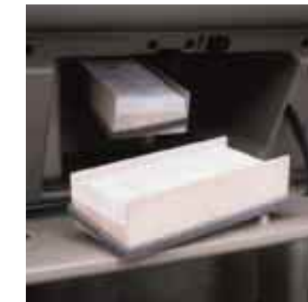
Venture's standard pollen filter elements are located at the rear of the glove compartment, so they're easily replaced when necessary.
