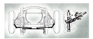
The integral type power steering assembly consists primarily of a gear reduction unit (recirculating ball and nut type), a power cylinder, and a hydraulic servo-control valve. A torsion bar between the steering shaft and valve spool assembly provides the driver with a positive feel of control.
