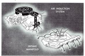
The intake manifold on the 410 cubic inch engine is water warmed assuring a more even stabilization of the fuel-air mixture. The location of the four barriel carburetor in the center of the manifold allows a short, nearly equal passage to each cylinder.
