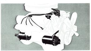
The high output capacity generator, located at the lower right front of the engine, adequately meets the electrical system demands, plus supplying a reserve for battery charging requirements.
