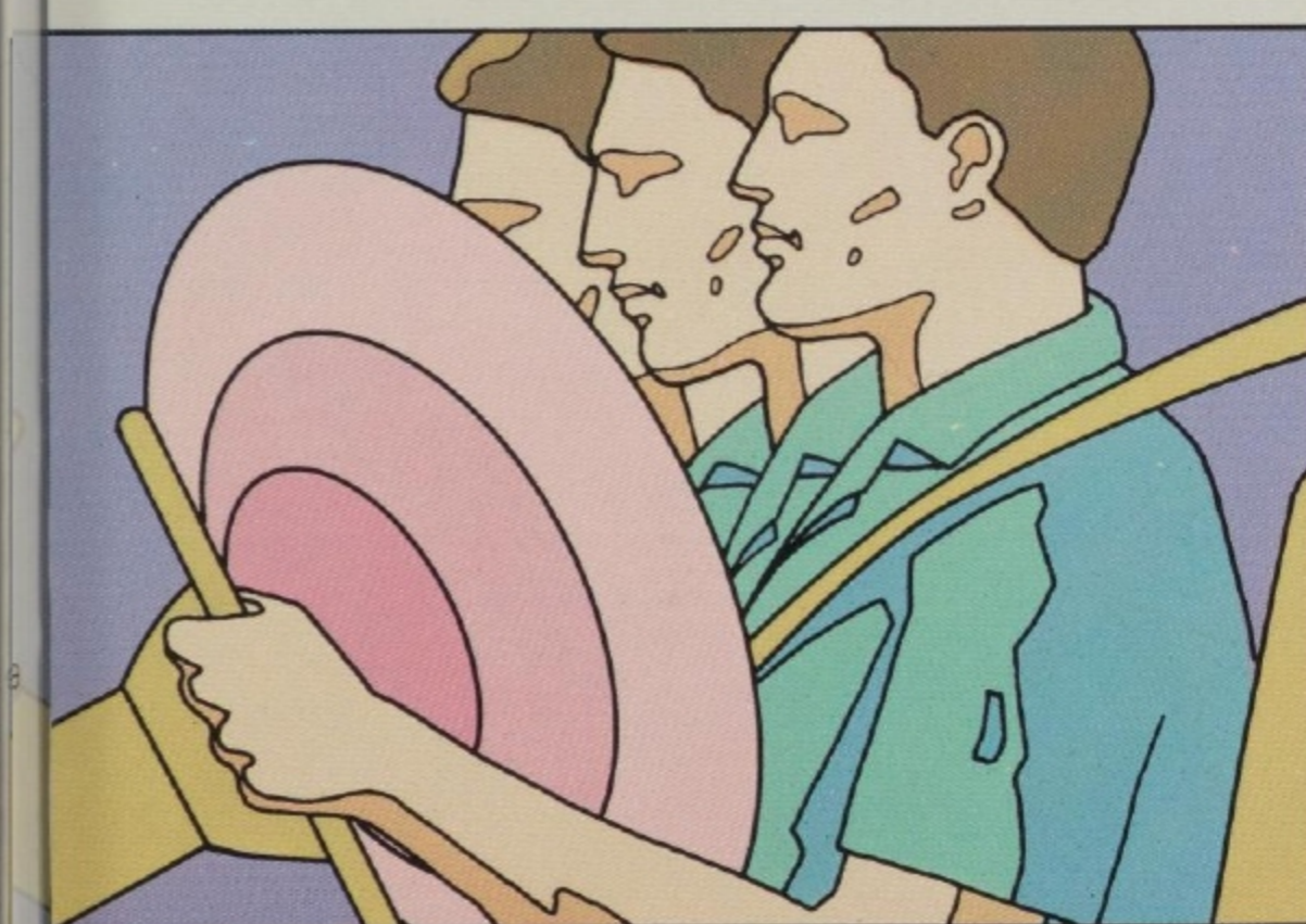
Air bag inflates in approximately 40 milliseconds.
