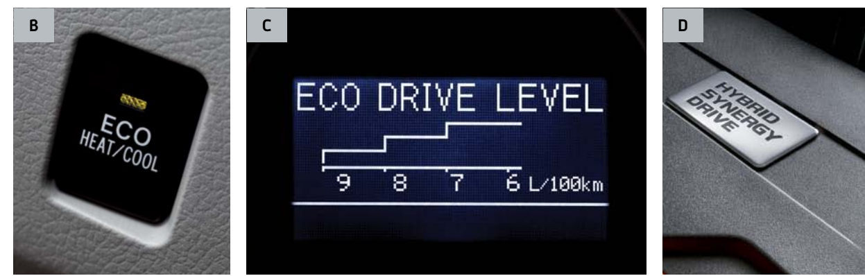
A. The multi-information screen shows how Hybrid Synergy Drive manages the flow of energy in your Camry Hybrid. B. Manual ECO mode conserves fuel by reducing energy used by heating and air conditioning. C. Optitron gauges with ECO Drive Level show current fuel economy while driving. D. Inverter cover - Part of Hybrid Synergy Drive's Power Control Unit is an inverter that transforms direct current supplied by the battery to alternating current used by the system to turn the electric motor and for use in the generator.
