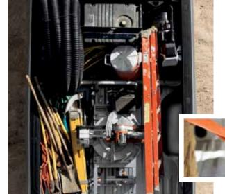
AVAILABLE CLEATS AND TIE-DOWNS Connected to the upper rail of the bed, the system uses four cleats rated at 100 kg (220 lbs) per attachment to help ensure that what's in the bed stays in the bed.
