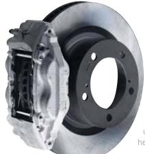
BIG VENTILATED DISC **BRAKES.** Front and rear (74 square inches of swept area, with 4 pistons in front) ventilated disc brakes quickly and effectively shed the extreme heat that builds up when hauling or towing the heaviest cargo.
