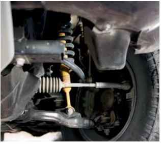
**BILSTEIN SHOCKS AND VENTILATED FRONT DISCS** Available Bilstein shocks take the edge off the bumps while the ventilated front discs help with sure stops.
