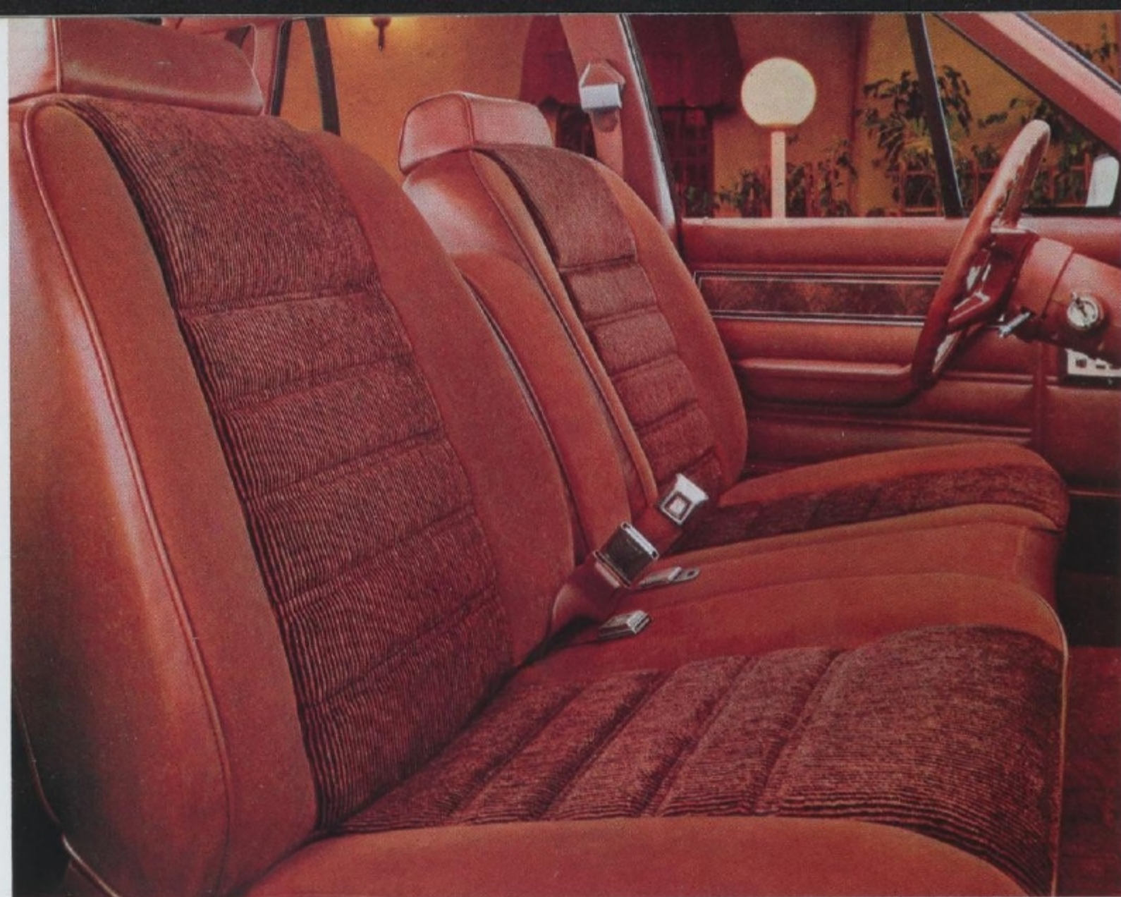
ZEPHYR GS Flight Bench seat, with fold-down center armrest, in Vaquero cloth.
