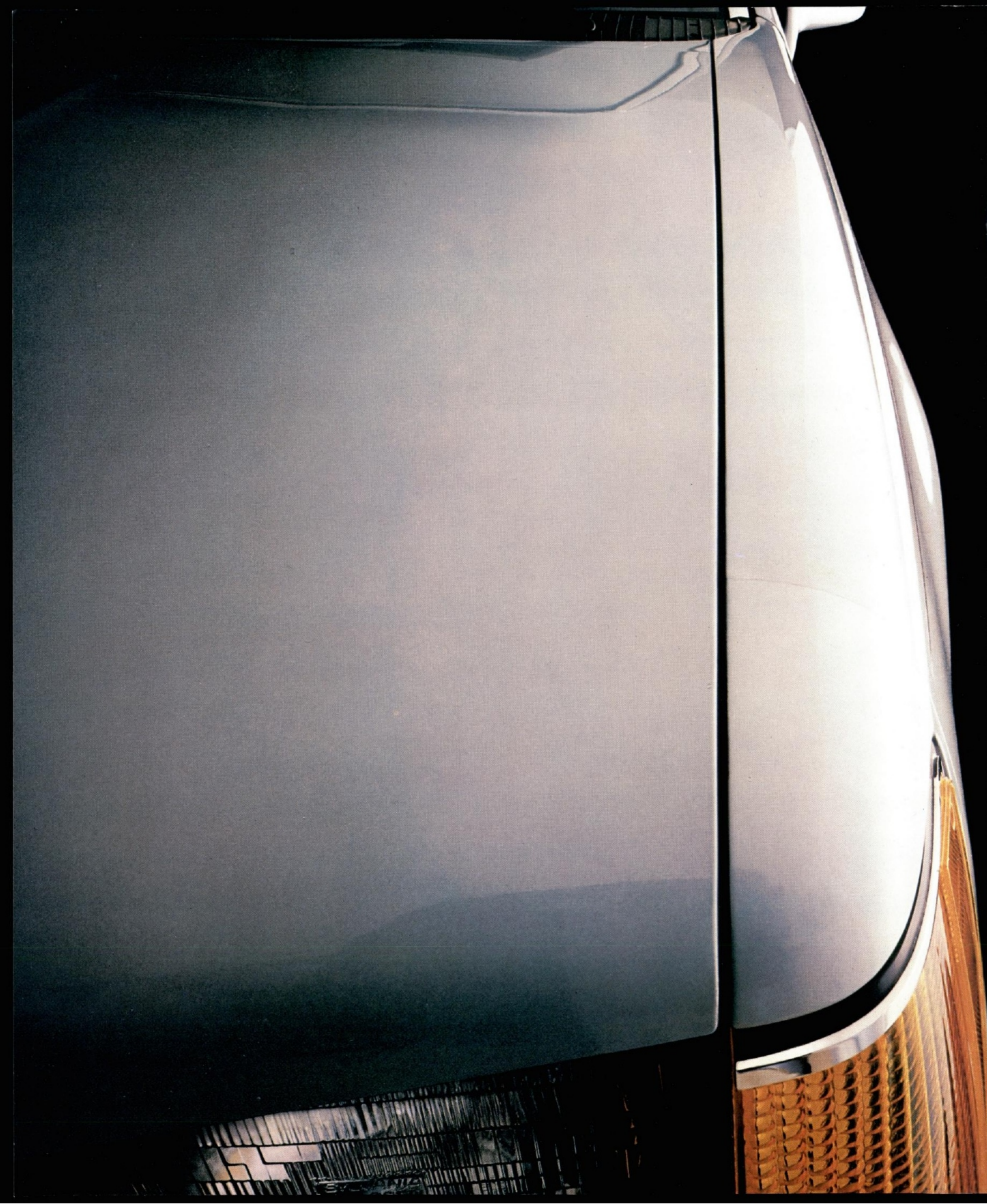
Statistical process controls and sophisticated gauges help keep the fit of Topaz body panels—such as this fender/hood seam—within \pm 1.5 millimeters of design standards.
