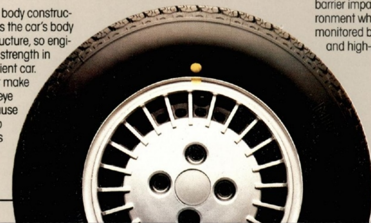
Matching the inherent high and low points of both tires and wheels helps give Topaz increased ride smoothness. This process is called tire/wheel indexing.
