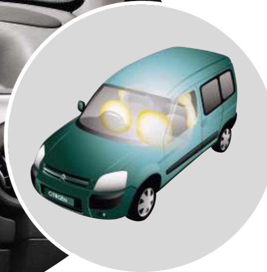
The Berlingo Multispace is fitted with both driver's and passenger's airbags as standard. To ensure extra protection, 18-litre side lateral airbags are also fitted as standard.
