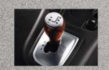
SensoDrive gearbox<sup>†</sup> allows you a choice of driving style – manual or fully automatic. Reacting faster than the most experienced of drivers in just a fraction of a second, manual gear change can be operated either by fixed column mounted paddles located behind the steering wheel or by the floor mounted gear lever with a forward and back movement.
