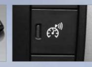
A clever control<sup>†</sup> located on the central console enables you to register a maximum speed. In the event of exceeding this preprogrammed limit, an audible warning will alert you.
