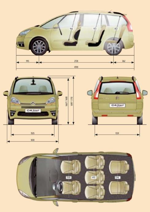
All measurements in millimetres
