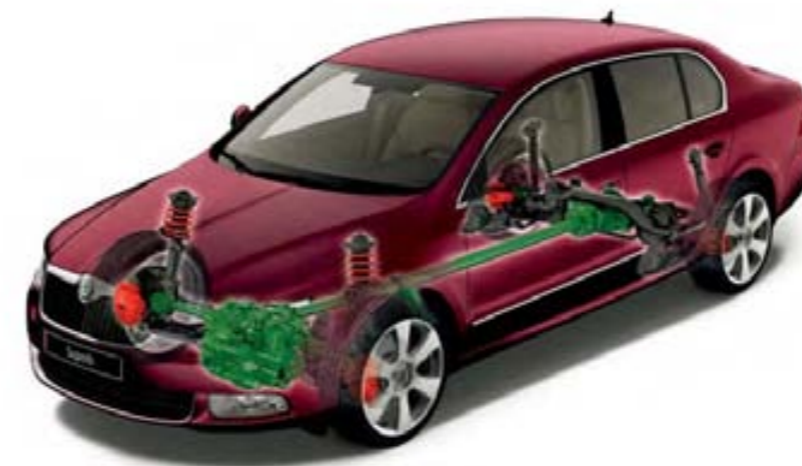
Superb with a 4-wheel drive and a 4th generation Haldex clutch (1.8 TSI/118kW; 3.6 FSI V6/191kW and 2.0 TDI CR DPF/103 and 125kW engines)
