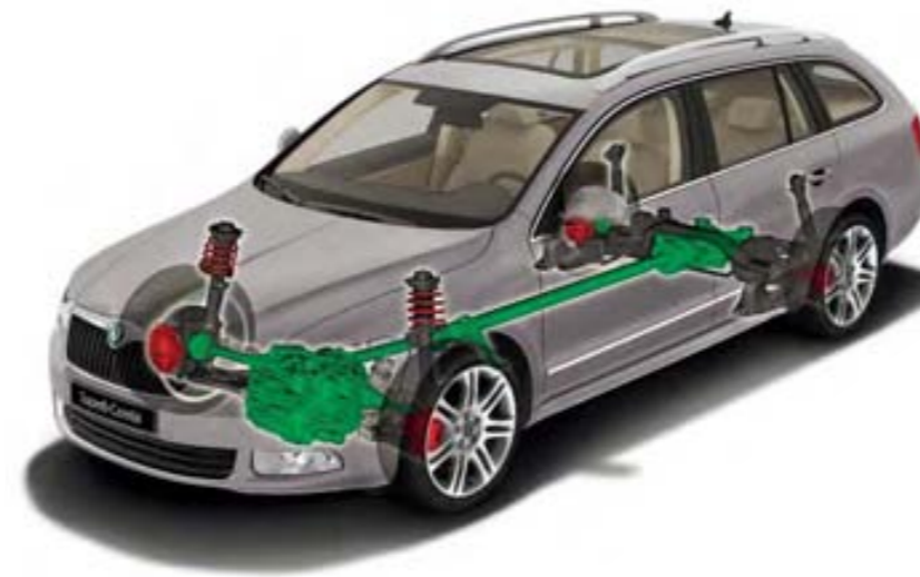
Superb Combi with a 4-wheel drive and a 4th generation Haldex clutch (1.8 TSI/118kW; 3.6 FSI V6/191kW and 2.0 TDI CR DPF/103 and 125kW engines)
