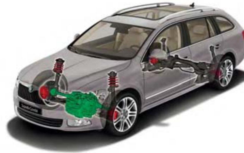
Superb Combi with a front-wheel drive (available for all engine versions except for 3.6 FSI V6/191kW engine)
