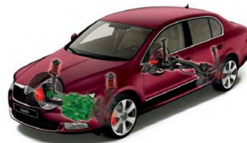
Superb with a front-wheel drive (available for all engine versions except for 3.6 FSI V6/191kW engine)
