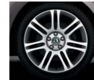
7.5J x 18" Themisto alloy wheels with a polished surface for 225/40 R18 tyres.
