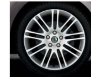
7.5J x 18" Luxon alloy wheels with a polished surface for 225/40 R18 tyres.
