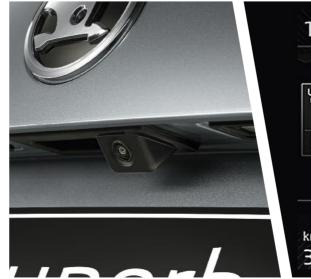
Enjoy easier parking by equipping your car with the rear-view parking camera, which is located on the handle of the boot. It monitors the space behind the car and indicates the driving lanes, based on the vehicle width.
