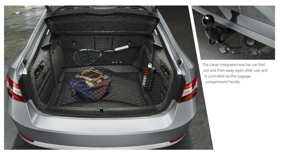
The boot net programme increases the flexibility of the luggage space while tightly securing objects. It includes one horizontal and two vertical nets.
