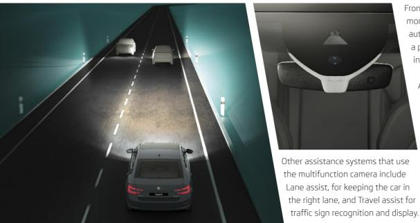
Now you can use high beam for longer without blinding incoming traffic. The Smart light assist can not only switch between the lighting functions but can also dim the high beam, using a multifunction camera located behind the rearview mirror.
