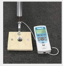
Testing of fixing element strength
