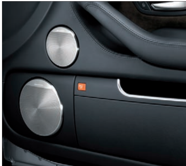
Speakers, part of Bang & Olufsen Advanced Sound System
