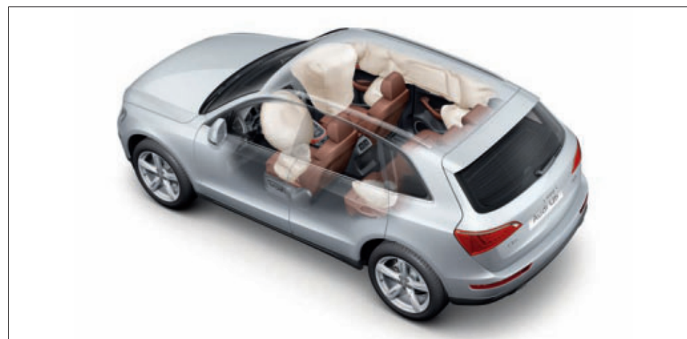
Standard side airbags for driver and front passenger seat, plus rear side airbags
