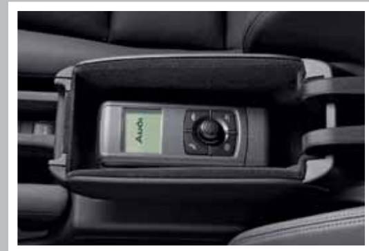
Remote SIM Access Profile Bluetooth adaptor cradle
