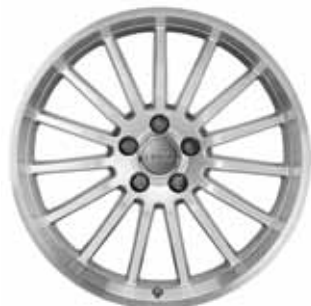
18" x 7.5J '15-spoke' design alloy wheel, Part number: 8P0071498666
