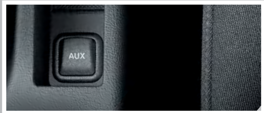
AUX-IN socket in front centre compartment (standard on Concert and Symphony radio)
