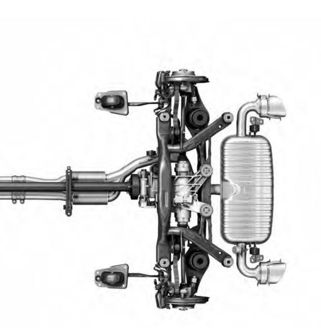
In the Audi A3, quattro® all-wheel-drive continuously distributes drive power between the front and rear axles depending on weather conditions, road surface and gradient, which increases flexibility for an enhanced, sportier drive.
