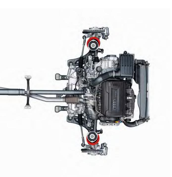
In the Audi A3, quattro® all-wheel-drive continuously distributes drive power between the front and rear axles depending on weather conditions, road surface and gradient, which increases flexibility for an enhanced, sportier drive.
