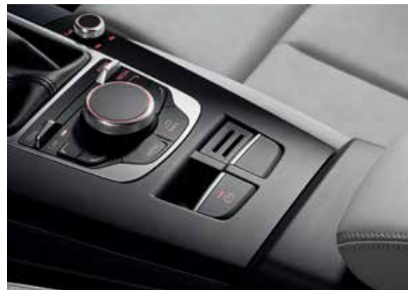
Electromechanical parking brake and MMI control panel
