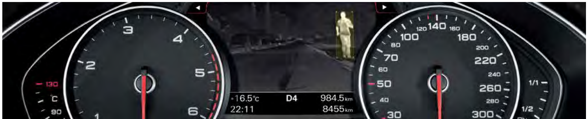
Night vision assistant with pedestrian detection
